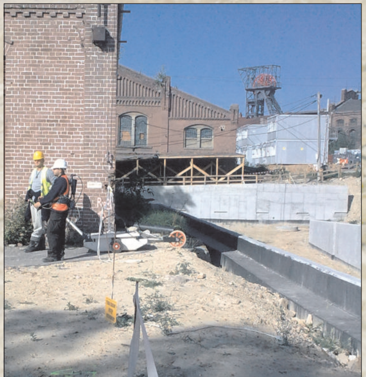
▲ Georadar profiling method for the determination of shear planes in the ground in the former coal mine area
