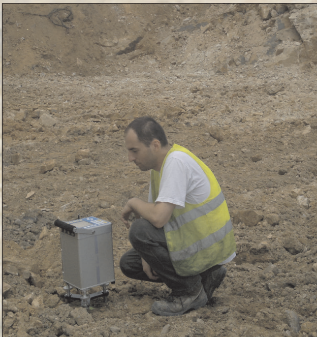
▲ Microgravimetric survey to locate the wandering voids being the result of shallow mining
