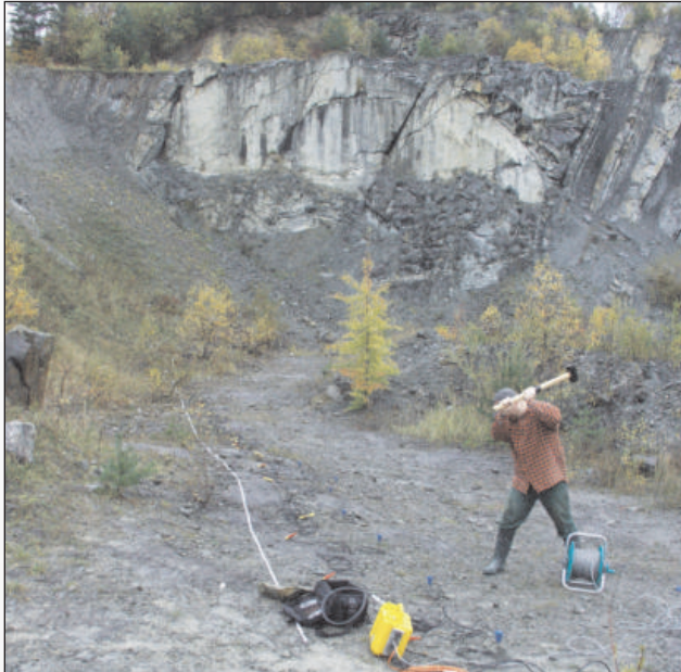
▲ Engineering seismic surveys to determine the thickness of the weathered layer in sandstone quarry
