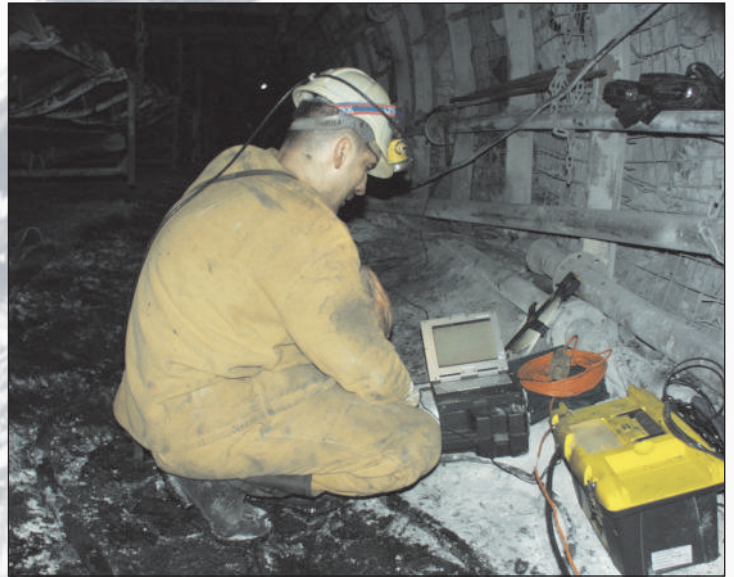
▲ Seismic measurements to assess the risk of rockburst in hardcoal mine
