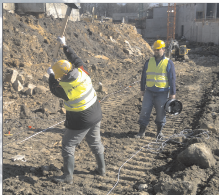
▲ MASW seismic survey to detect cracks and loosened zones in post-mining area
