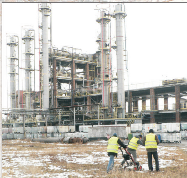
▲ GPR acquisition in the chemical plants in order to identify the old foundations remnants, unknown infrastructure, fuel tanks, performed for the new investment. Study was conducted using modern biantenna georadar system, in a dense grid of profiles to get appropriate vertical and horizontal resolution. This is very important for mutual verification of detected georadar anomalies.
