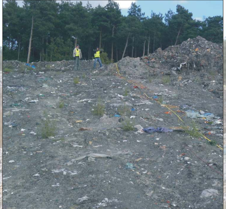
▲ Seismic measurement on municipal wastedump place in order to identify the boundaries of layers and the range of wastes
