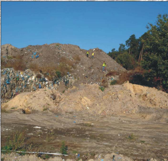
▲ Seismic measurement on municipal wastedump place in order to identify the boundaries of layers and the range of wastes
